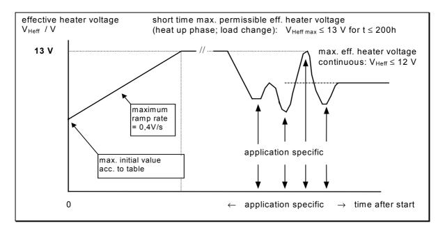
Maximum permissible heat up rate with limited heater power to reduce the thermal stresses in the heat-up phase
